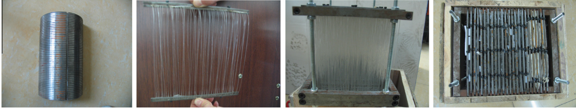
Fig. 2. Fastening method and casting mold (Method 2).
